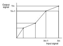
Adjustment range: (Common to output-1 and output-2) Input adjustment: ±1% of span or more (Zero/Span) Output adjustment: ±5% of span or more (Zero/Span)
