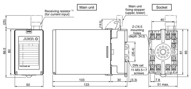
\*1: "250  $\Omega$ " or "100  $\Omega$ " is attached for current input.
